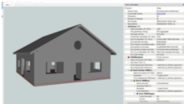
FZK Haus (known from IFC lecture) converted into CityGML by FME; building elements are visualised. Source: GitHub - tum-gis/ifc-to-citygml3: An FME workspace for converting IFC data sets to CityGML 3.0 data sets
